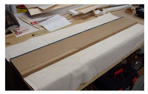
The aluminum angle is placed against the factory cut edge of the MDF, clamped and 6 evenly spaced (about  $7 \frac{1}{2}$ ") holes drilled using a 5/32" bit, deep enough so the #10 screws will not bottom out. The aluminum is removed and drilled to 3/16" for clearance and the holes in the MDF tapped to the correct thread. Locate the angle and install the screws and the fixture is ready for action.
