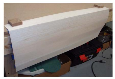
When all the joints are glued wipe off the excess, cover with wax paper and weight down the balsa sheet. The weight will keep the sheet flat and give you a better joint. Take care to weight the edges or they will curl and the joint will open. Let it dry for about 20 minutes before lightly sanding the side that is not taped. After about 1hr. carefully remove the tape, wipe any excess wet
