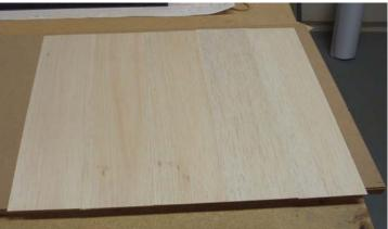
After matching all the sheeting, align and tape the joints on one side with blue painters tape. The tape will act as a hinge to open the joint but does not pull the fibers from the wood when removed like regular masking tape will.
