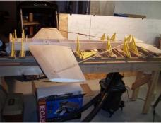
plane the same as we have always done but by using 2 rigid pieces we can move the wing into perfect alignment without going back and forth to
