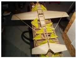
The idea is measure from a point near each wing tip usually on the wing spar to a point on the center line of the fuselage near the tail of the
