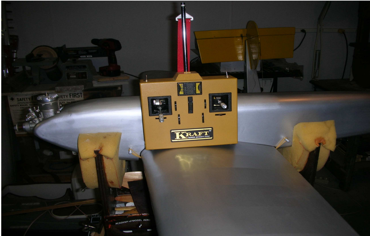
Taurus with Kraft Series 79 two stick radio and Veco .61
