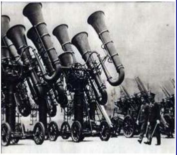
I bet none of you ever saw anything like this before. No, it is not the horn section of the Imperial Japanese Army Marching Band. This is how air attacks were detected before the invention and use of radar...
