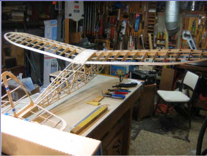
Roger Smith with his Quaker Flash sporting an OS FS .20, three channels for guidance and Solartex for covering. Looks good, outstanding workmanship.
