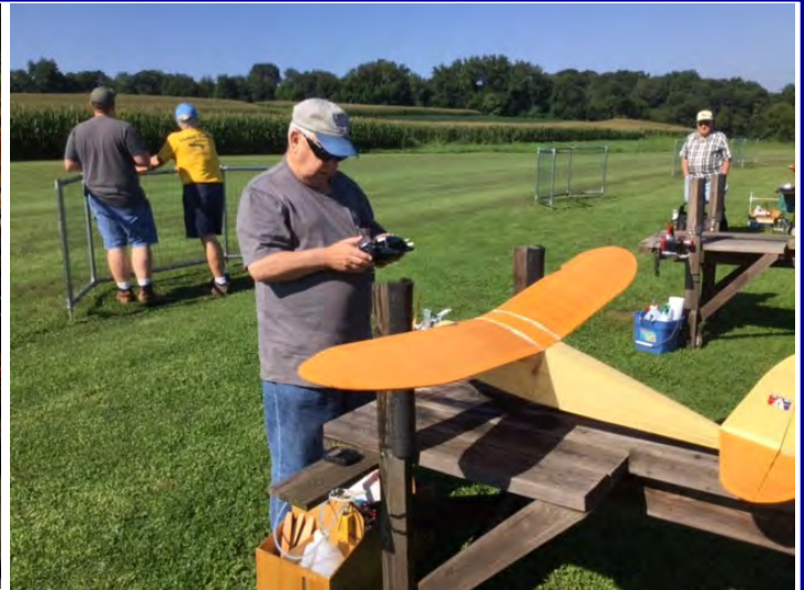
Roger Smith with his Quaker Flash sporting an OS FS .20, three channels for guidance and Solartex for covering. Looks good, outstanding workmanship.
